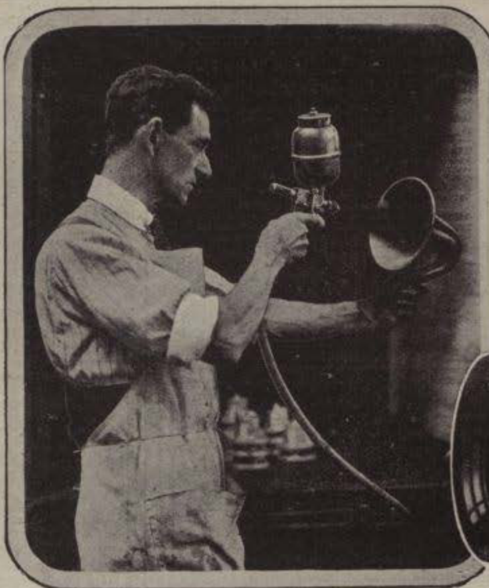
Illustration showing the horn of a Brown Loud Speaker being sprayed with enamel.
